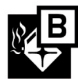
Class B Fires: Fires involving flammable Liquids such as petrol, diesel, greases, paints etc.
