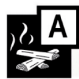
Class A Fires: Fires involving organic solids like paper, wood, textile etc.
